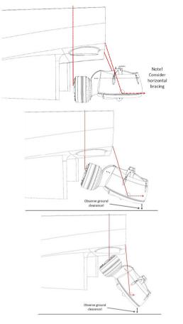
Figure 3.2-9 Lifting and up-ending thruster
