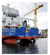
Remove:Install:Rudder with steering gear•PMazm includingNozzle with propellersteering gearShaftline•Lubrication systemsGear•Helicon- controlElectrical motorsystemFrequency converter•Frequency ConverterBridge control system•HEMOS
