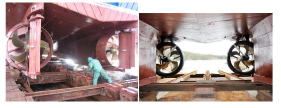
Propulsion system : 2x500kW, 440V 60Hz "Classic diesel electric Length: 31,25m Breath: 9,6m
